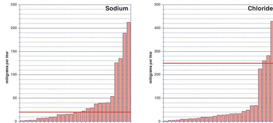
Distribution of sodium and chloride concentrations in all sampled wells. Red lines represent maximum acceptable concentrations.
