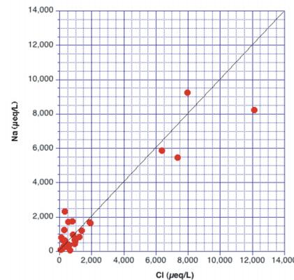
Scatter plot of sodium versus chloride. Points above 1 to 1 line indicate secondary sources of sodium while points below line indicate either Calcium chloride or exchange reactions that remove sodium
