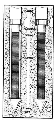
Figure 4: Sandpoint Installed with Protective Oversized Casing. During Driving, the casing pushed a special heavy duty drive point downward while the casing protects the screened portion of the wellpoint. The screen is exposed at the predetermined depth either by driving it with an inner casing inserted through the oversized casing or pulling back the oversized casing (Driscoll, 1986).
