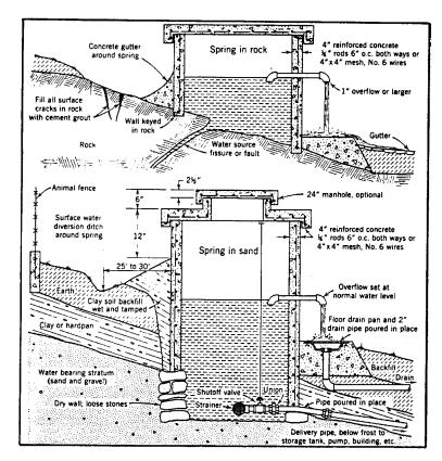
Figure 1: Properly Constructed Springs (Salvato, 1958)
