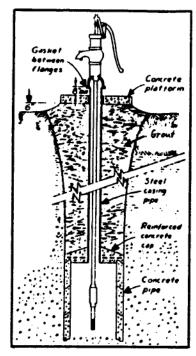
Figure 6: Dug Well Constructed with a Buried Slab
