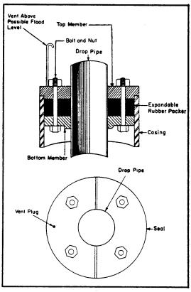
Figure 12: Detail of Acceptable Well Cap
