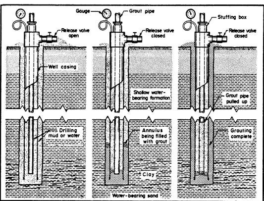
Figure 10: Grout Installation by Positive Placement Interior Method with Capped Casing (Pressure Grouting). Pressure is maintained until the grout hardens. (Johnson 1966)
